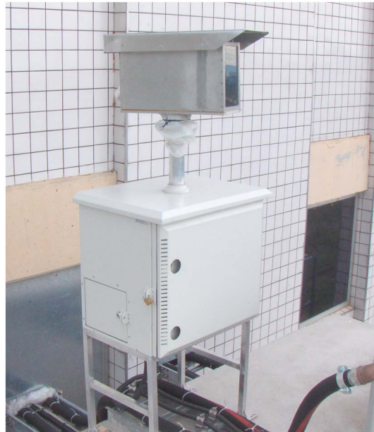
Figure 1. A RAMMER sensor (Phantom high-speed video camera on top with protective box for data computer below) located at site 2 (Vanguarda TV station tower).
